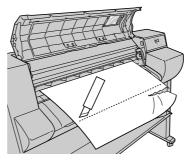
**6** Open the tray, pull the tray open lever, then pull out the roll media tray.
